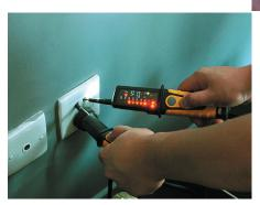
The most simple and easy to use voltage detector that is a must for all technicians. Not only does it measures and dectects voltage, it also determines phase rotation directions.
