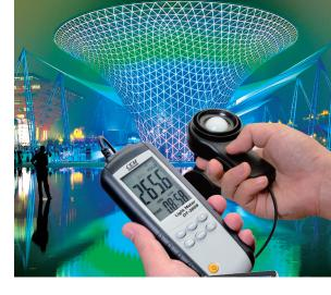
The data logger is designed for logging and measuring Light intensity for projects, quality control, health control and measuring Light intensity of various kind of environments like factory, school, office, transportation line, and so on.
