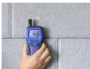
Measure moisture of wall material with non-invasive Pinless technology
