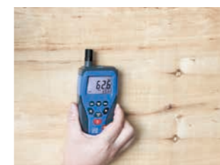
Pinless moisture measurements
