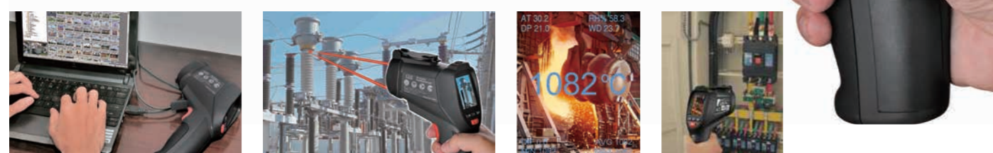
Upload images and videos to a PC or laptop for further analysis or use for report documentation. Dual laser targeting & D:S = 50:1 Fold reading on the images High accuracy (1.0%) measurement
